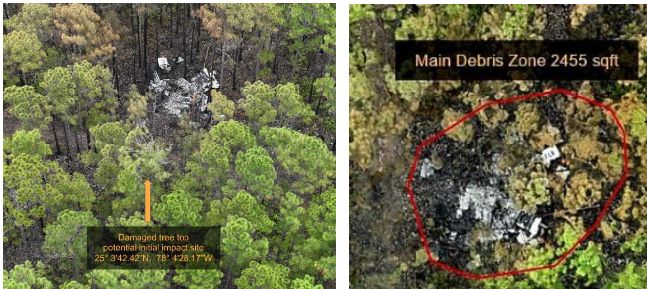
Fig. 6: (Left) drone view of aircraft initial point of contact; (Right) drone view of main debris zone
