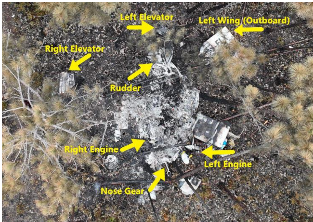
Fig. 7: Distribution of C6-FLX wreckage at crash site
